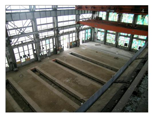
Figure 2 Vacant Erecting Shop Today – Note Intact 250 Ton Overhead Crane
